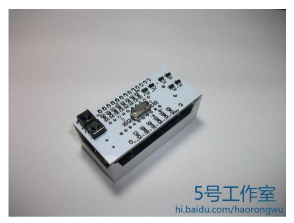
Then the two micro-switches are welded to the top, as shown above. Check all the devices have no gaps, then the digital pipe welding after we go up, or if the welding of the digital control, found that the device slightly less trouble, they must be checked before the next step.
