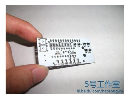
Using the same method to 6 SMD transistor welded to the top, R9: 20K (marked 203), R10-R14 (marked 102); and the base resistance and capacitance oscillator circuit 30PF welded on top, complete after as shown in Fig.
