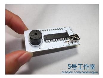
Then you can cut crystal pin microcontroller soldered, pay attention not to engage in anti-MCU position, the semi-circle above the corresponding PCB footprint microcontroller semicircle above, after the buzzer with 1uf active filter chip capacitors are soldered above (clear plastic strip packaging, welded to the C3 position).
