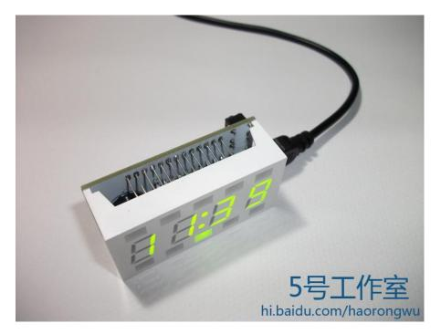
Access mini-USB cable to use as a power supply voltage output is 5V. Initialization time is 12 o'clock, you will hear the buzzer sounding cry with digital flicker up and down the grid, to remind the whole point of arrival.
