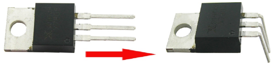
① Bend the pin 90 degrees
