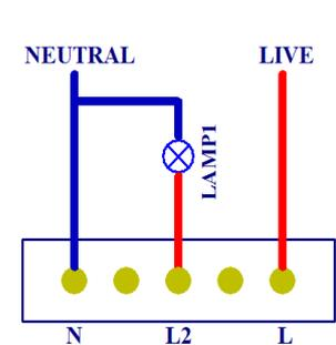
A switch wiring diagram
