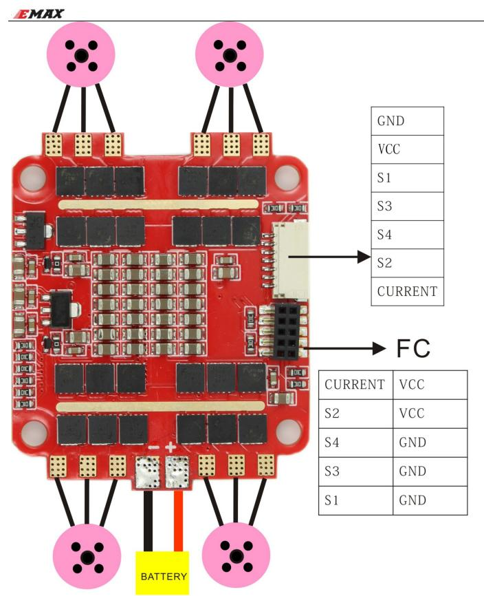
Note: Please be careful when soldering battery lead to prevent short circuit!
