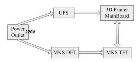
2. When system fails to connect with power, outage detection module will inform touch screen automatically and enters into printing suspending status. Power supply of UPS will depart printer head from model.
