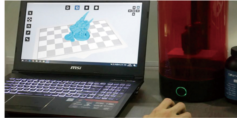
Step1: Add STL file model to SparkStudio to add support and slice
