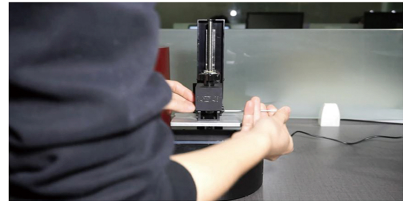
Step3: Level platform when first print (No need to level again next time).
