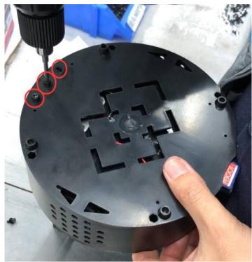
$2. \ \mbox{Remove the resin tank and loosen six screws on the panel top (remember to collecting the falling nuts).$
