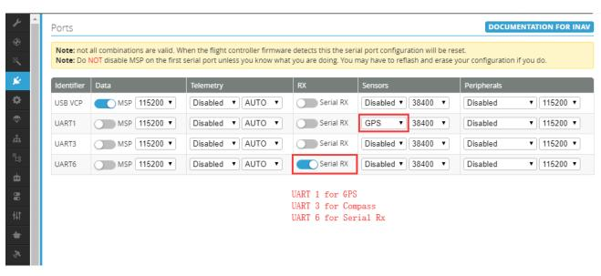
GPS is pre-solder to UART 1, Compass is pre-solder to UART 3, please enable GPS for UART 1.
