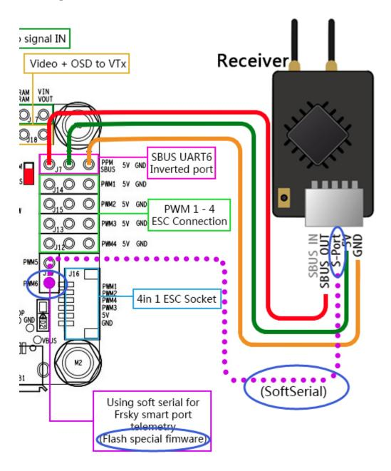
Then enable the softserial feature on the configuration tab.
