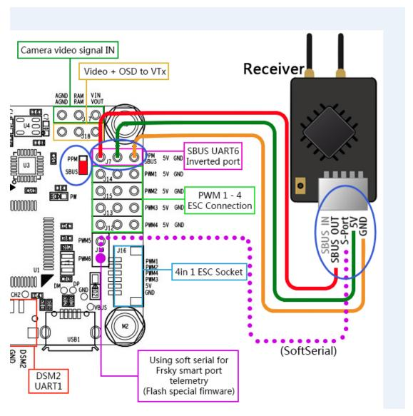
Sbus receiver/Ibus receiver/PPM receiver please enable Serial RX for UART6
