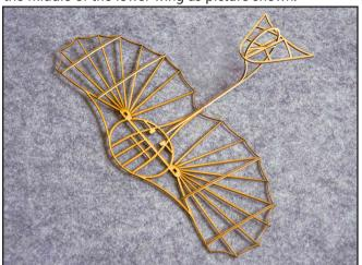
2.Glue the 8pcs ribs of the upper and lower wing as number marked out, make sure they are parallel to the middle bracing of the wing, which could slightly bent to curved shape.
