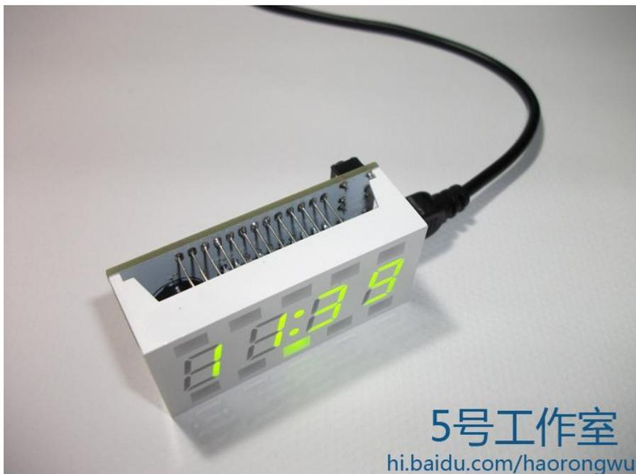
Access mini-USB cable to use as a power supply voltage output is 5V.
