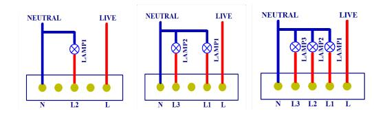
A switch wiring diagram
