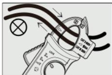
DC current mode, due to the existence of electromagnetic field, please push ZERO button 2S, set the value of display to zero. Keep the direction of the meter and zeroing in line.
