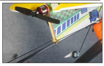
16.Install the battery with magic sticker, bind all wires, receiver, ESC and other accessories.
