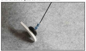
10. Assemble the motor on the motor mounting board and stick it on the tail of fuselage as shown.
