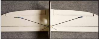
8.Stick 5\*100mm carbon plate on the tail of fuselage. Reinforce the vertical tail with 1mm thin carbon rod, keep vertical.
