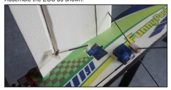
15.Insert 2pcs 435mm length carbon rod from the two spacing holes of the bottom of motor mounting board. Install the aileron servo with the same way like installing the pull rod of elevator servo and rudder servo.
