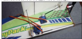
12. Stick the aileron servo, assemble the "Z" type steel wire on the second and third hole.
