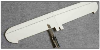
5. Stick the horizontal tail and vertical tail on the tail of the squared carbon tube as shown.
