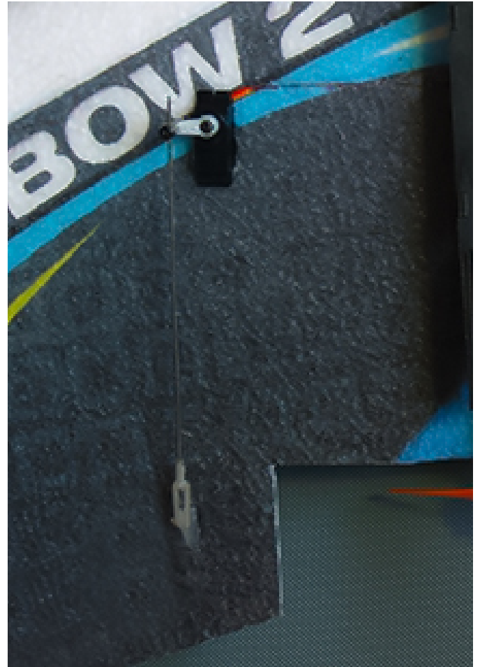
0.03 Make a connecting rod by using the Z-type steel wire and carbon rod, and then connect the servo and aileron.
