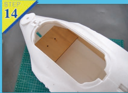
Fig13-14: Joint the left and right side of fuselage together as figure
