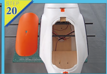
Fig19-20: Install relative components in the fuselage and canopy hatch
