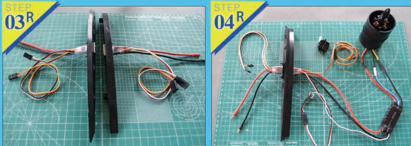
Fig3-4: Connect well servo on the right wing, ESC and motor. (Attention: Link the same color of connection wires together, such as servo, ESC. The right wing motor turning connection method.)
