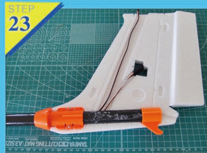
Fig23-24: Install and fix the vertical stab, extended wires, plastic parts, 3K carbon fiber tube. (Attention: The long wires connect with elevator, the short wires connect with rudder.)
