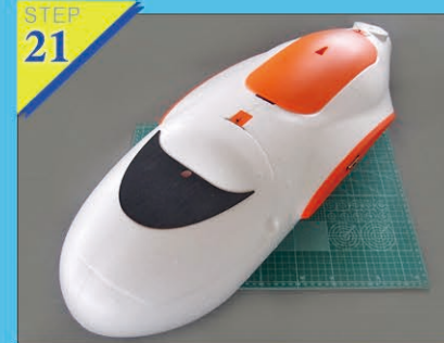
Fig21-22: Install layer at the bottom of fuselage
