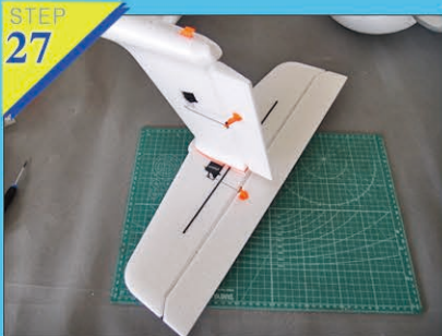
Fig27-28: Connect well the horizontal stab with vertical stab, fix 3K carbon tube on the fuselage by 3 screws(2.5mm)
