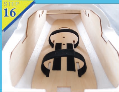
Fig15-16: Adhere cable ties and velcro tape into the fuselage
