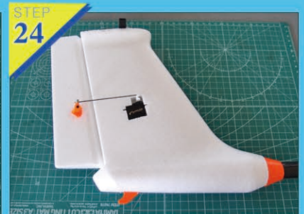
Fig23-24: Install and fix the vertical stab, extended wires, plastic parts, 3K carbon fiber tube. (Attention: The long wires connect with elevator, the short wires connect with rudder.)
