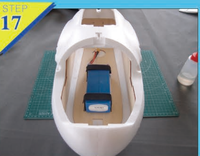
Fig17-18: Adhere the plastic part on both side into the fuselage
