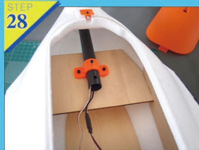
Fig27-28: Connect well the horizontal stab with vertical stab, fix 3K carbon tube on the fuselage by 3 screws(2.5mm)
