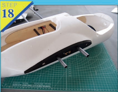
Fig17-18: Adhere the plastic part on both side into the fuselage
