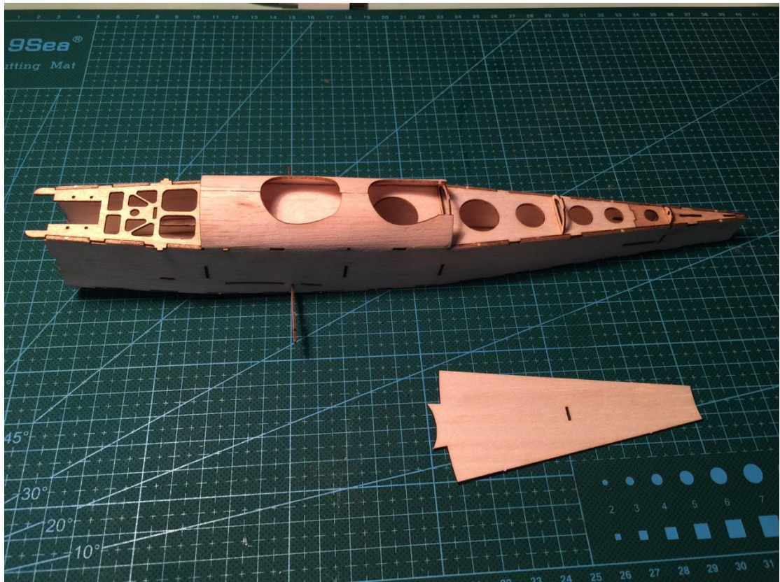
6、 The fuselage mask is bent from the both side to the center, forming the fuselage surface. This step should be done with care and a wet cloth can be used to wipe out the board to reduce the possibility of fracture during the bending.
