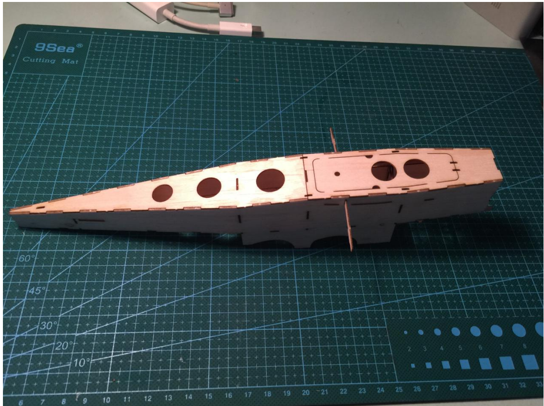
6、 The fuselage mask is bent from the both side to the center, forming the fuselage surface. This step should be done with care and a wet cloth can be used to wipe out the board to reduce the possibility of fracture during the bending.
