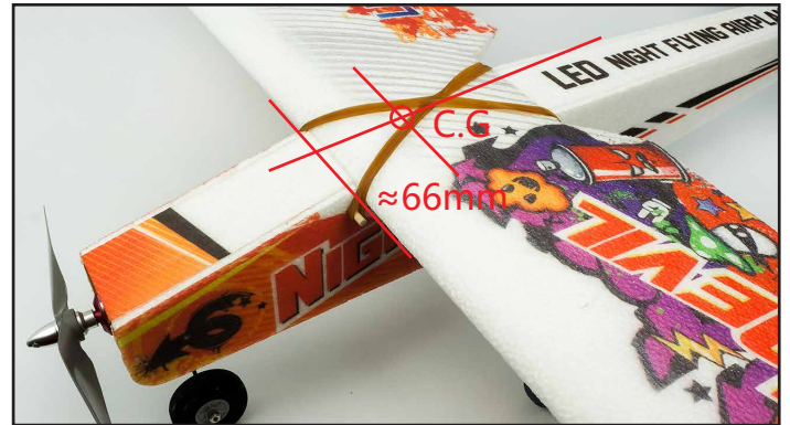
Adjust the C.G, C.G is 66mm from the leading edge. Then start your flight.
