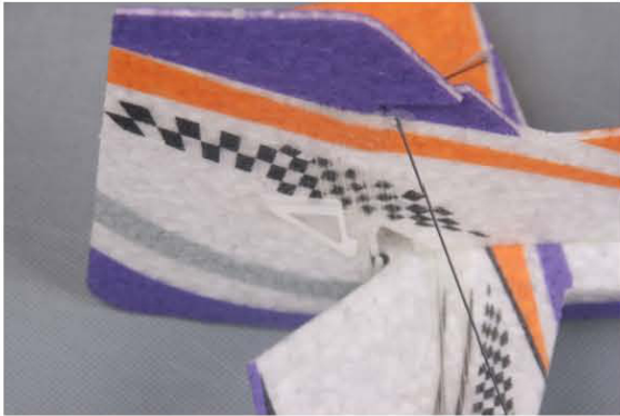
Install the rudder control horn, same as above steps.
