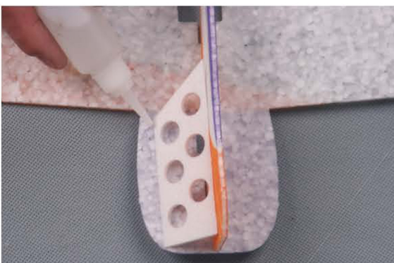
Glue the horizontal and vertical fuselage doublers to the underside of the horizontal and vertical fuselage as shown.
