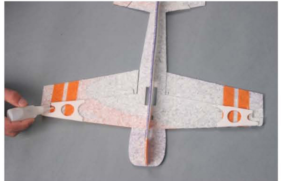
Glue the wing doublers to either end of the wing as shown.
