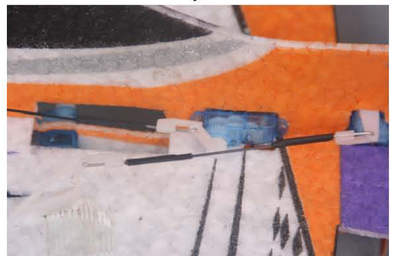
Secure one piece of wire to one end of the carbon rod, using one piece of heat-shrink material. The piece of wire should overlap the carbon fiber rod at least 1" (25mm). Heat the heat-shrink material with a heat gun to shrink it into place. PRO TIP For extra security, apply a few drops of glue to the end of the pushrod and allow it to "wick" into the joint.
