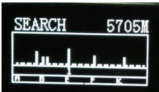
A typical searching result shows: there are 6 signals, and E1(5705M) is most strong. You can press confirm to select it, or you can up or down to select another channel and press confirm to show it,
